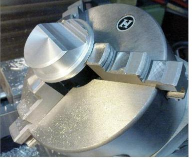
Complex parts such as this one, are produced on the tool milling machine in several working steps with an accuracy in the micro meter range ...mainly for the tangential tone arm
